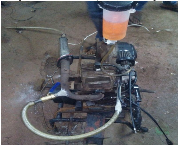
Fig. 1. Self-made EGR setup on two stroke engine.
